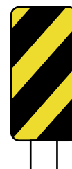
Reflector placed on the end-rails on narrow bridges or on other obstructions to make them stand out.
